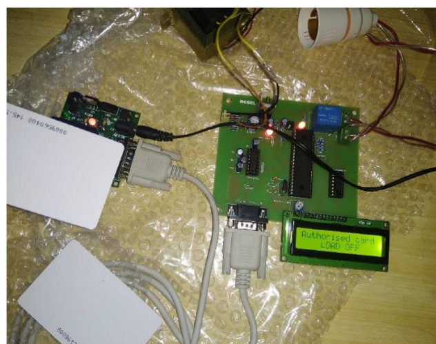
Fig10. View of authorized card LOAD OFF
